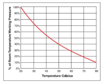
Example from the Celsius Chart If Working Pressure at 20°C is 14 bar, then the WP at 50°C is 14 x 40%, or 5.6 bar.
